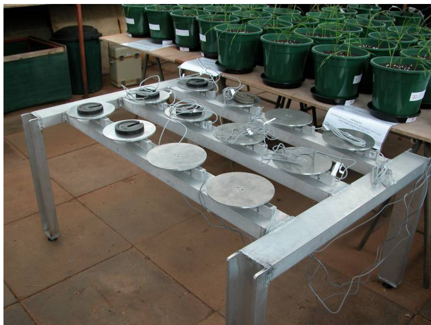
Figure 1. Electronic scale system used to measure evapotranspiration from each pot.
