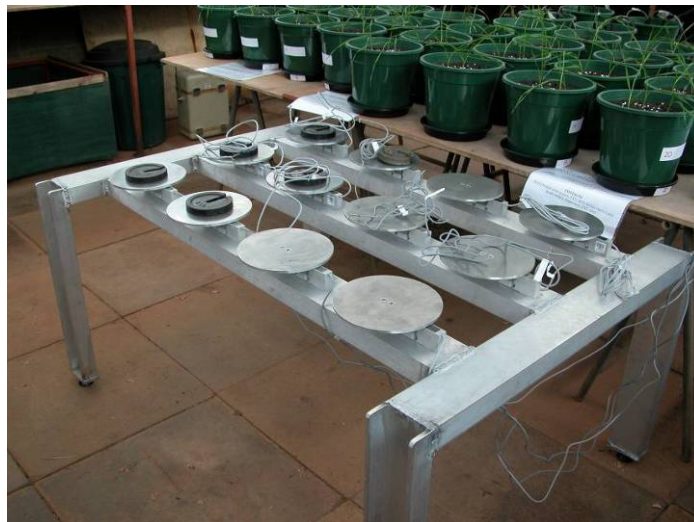
Figure 3. Electronic scale system used to measure evapotranspiration from crops in the glasshouse at the University of Southern Queensland (USQ), Toowoomba.
