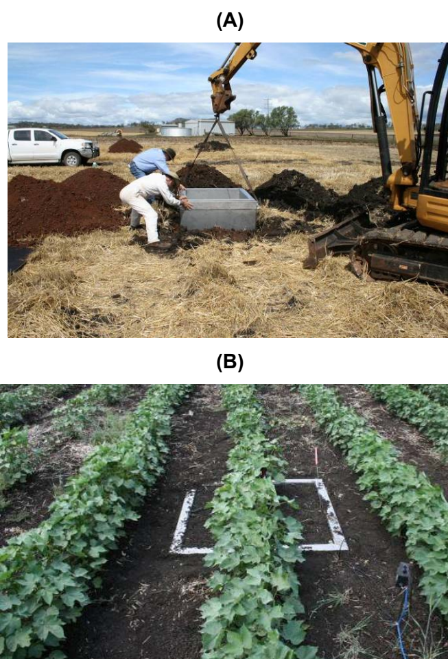
Figure 1. One of the lysimeters at Kingsthorpe (A) during installation and (B) planted to cotton in 2008-09.
