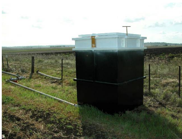
Figure 1. Lysimeter design 1 , Constructed of normal steel and the inner lysimeter box rests on two springs, which serve as a counterbalance for the dead mass. The load cells only need to measure the mass changes due to water loss rather than having to measure the total mass of the inner lysimeter box.
