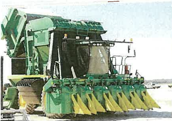
John Deere's new six row round module picker and baler on display at the front of the new gin
