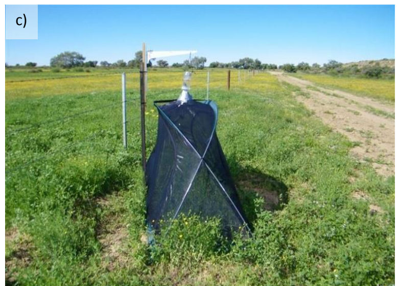
Fig. 13. First iteration of field emergence cages used in the Namoi Valley and inland Queensland. Fig. a) shows the detail on the capture mechanism, two plastic culture tubes glued together, with an ultraviolet LED wired into a solar-array that activated after dark. A 45mm powder funnel was attached to the bottom culture tube via the lid of the culture tube and a rubber washer. One-way glass fibre mesh prevented moths from escaping the culture tube. Fig. b) shows the offset cages that the capture mechanism was used in, at Boggabri NSW. Fig. c) shows how the capture mechanism was attached to the cages, via an iron post, tensile cord and metal bracket.
