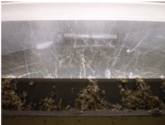
Figure 4 – (a) Top view of trash and fibre being removed by lint cleaner grid bars; and (b) bottom view, showing the access point where trash was collected beneath lint cleaner
