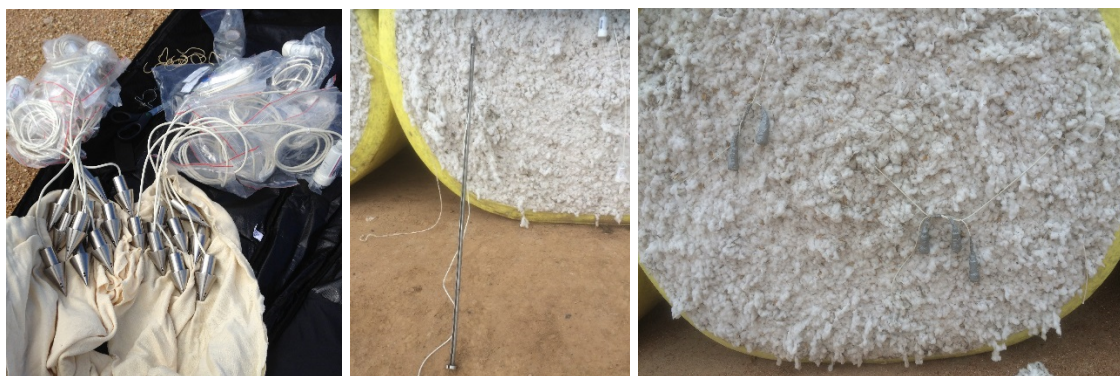
Figure 2. Temperature and moisture sensor with data logger for continuous monitoring of round modules.
