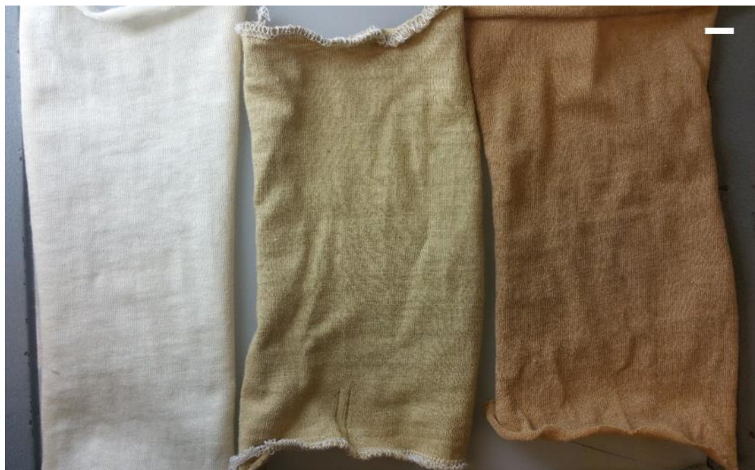
Figure 5.1. Experimental fabrics. Overlocked experimental fabric samples generated from white (left), green (centre) and brown (right) experimental cottons. Scale bar equals 1cm
