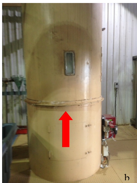
Figures 1(b) and 1(c) – Photos show position of IntelliGin system in a cotton gin; arrow in shows direction of air and cotton flow to battery condenser
