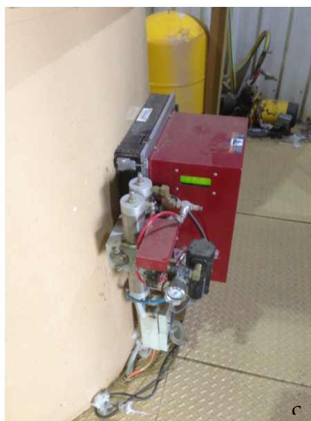
Figures 1(b) and 1(c) – Photos show position of IntelliGin system in a cotton gin; arrow in shows direction of air and cotton flow to battery condenser
