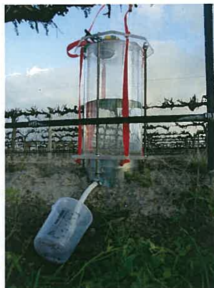
Figure 2. Cornell sprinkler infiltrometer during measurement of infiltration into soil mounded under the vines.
