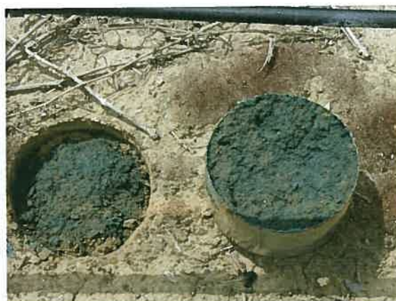
Figure 9. Horizontal distribution of dye tracer after infiltration of 32 mm of rainwater followed by 64 mm of dye solution.
