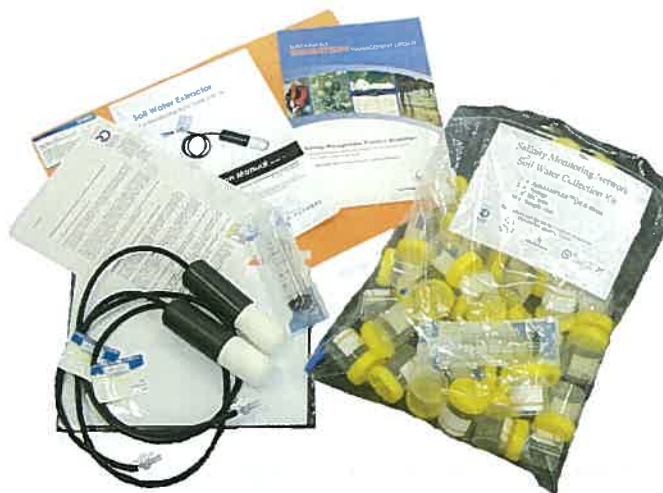
Figure 21. Salinity monitoring network support pack.
