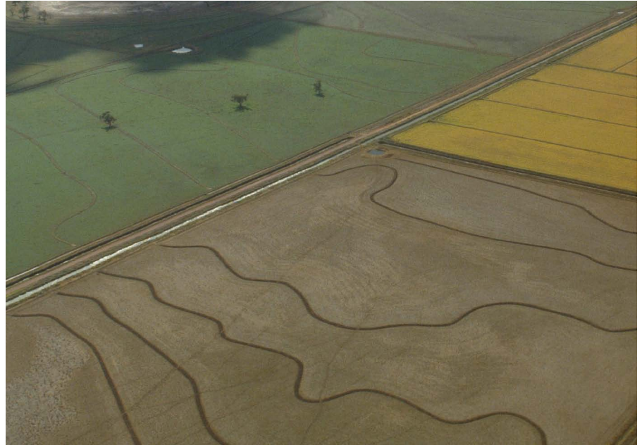
Figure 5.1.5. Bankless channel system commencing irrigation (Photo: M. Grabham)
