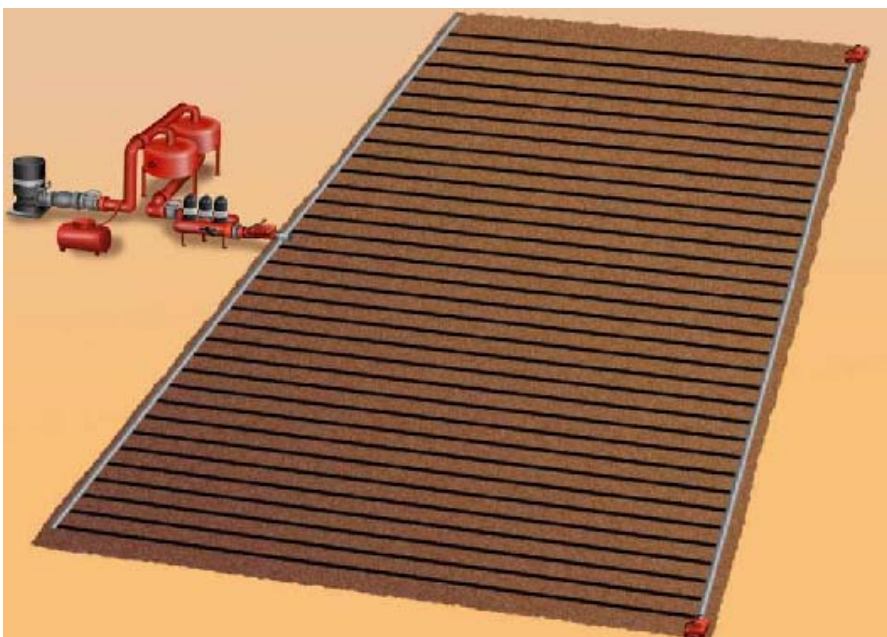
Figure 5.1.11. A typical drip layout (Netafim)
