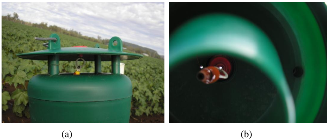
Figure 2.4. (a) side view of pheromone trap with pheromone lure hanging inside, (b) inside view of pheromone trap with pheromone lure hanging inside.
