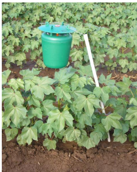
Figure 2.6. Pheromone trap placed above the cotton crop canopy by using flexible PVC electrical conduit pipe and strong wire.
