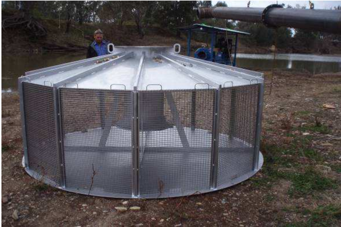
Figure 4. Experimental fish screen showing removable mesh screen panels. These could be removed and replaced with panels of different mesh size. Some were replaced with aluminium blanks to manipulate approach velocity.
