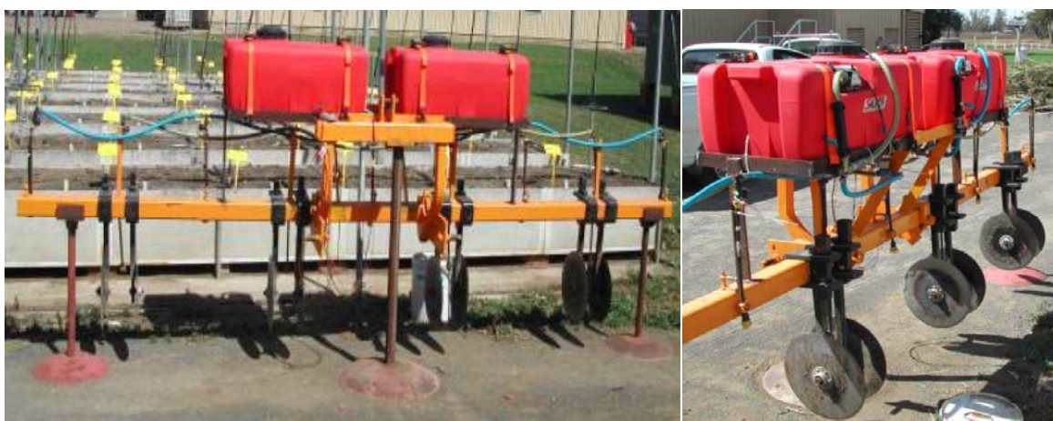
Fig. 25. Modified implement to simultaneously cut vetch runners and apply Sprayseed® to bed surfaces and Roundup® to furrows.
