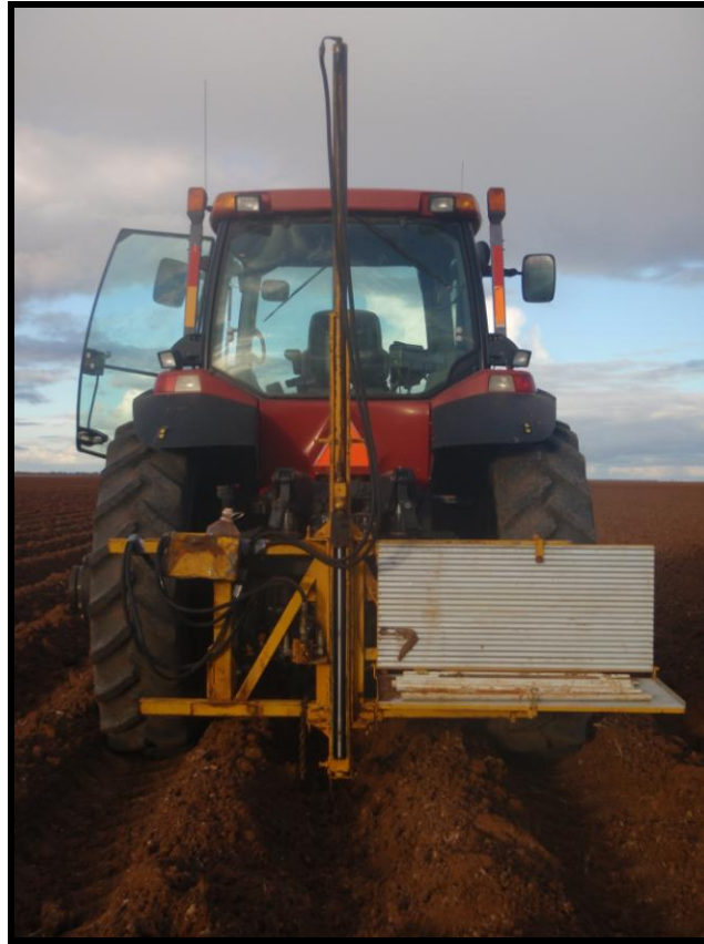
Figure 3.8. Single-stroke tractor-mounted hydraulic corer used for soil core sampling after 2.5 years
