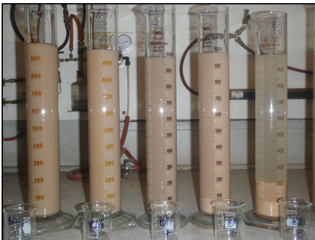
Figure 3.9. The measuring cylinder on the right contains Mount View (600-800 mm depth) soil for particle size analysis that was observed to flocculate after approximately 2 h, as a result of naturally occurring gypsum (1.35% total gypsum, Table 3.5)
