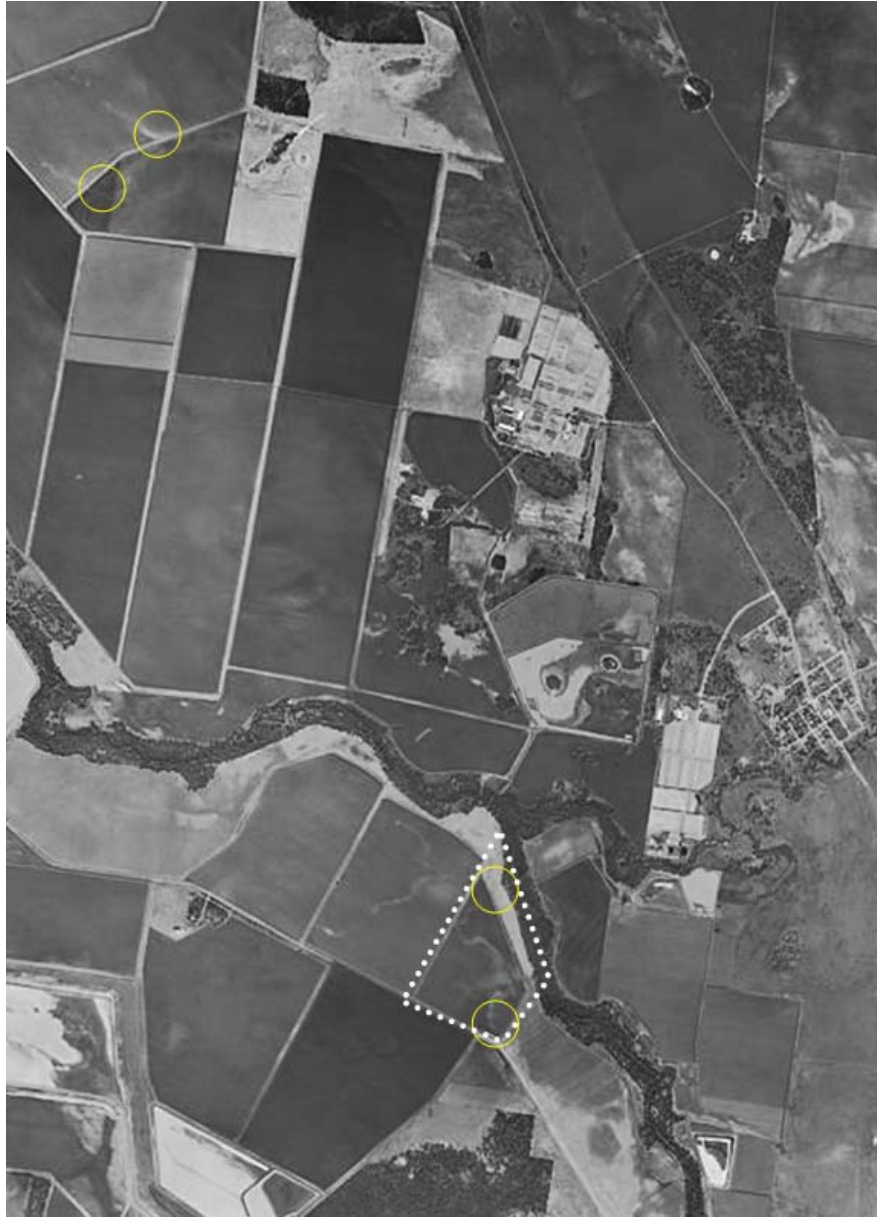
Figure 3.2. Aerial photograph showing a portion of Auscott’s “Midkin South” cotton farm. Circles indicate the areas near the field site where extensive water logging has been found. The study site is outlined. This aerial photo was taken during seed emergence and shows the disrupted emergence occurring in linear patches of bare soil above the palæochannels (pers. com Tim Richards, Auscott Farm Manager, May 2006).
