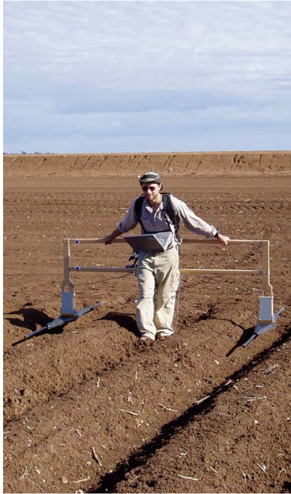
Figure 3.12. Self-contained ground-penetrating radar survey using the 50 MHz antennae in the common-offset orientation (two metre separation). The antennae were held at a constant height above the ground by attaching them to the backpack, which also held the harness-mounted laptop computer. The computer was used to adjust the survey parameters and view the raw data during collection.
