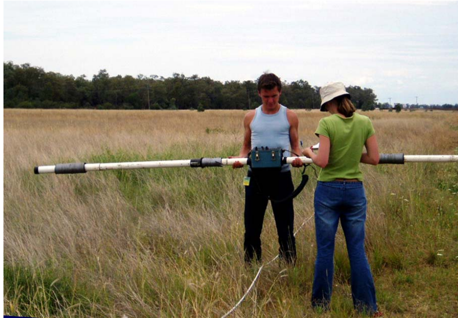
Figure 3.9. The Geonics EM 31 at 1 m above ground with dipoles vertically oriented during the survey the area of natural vegetation outside the paddock. The trees along the banks of Carroll Creek can be seen in the background.
