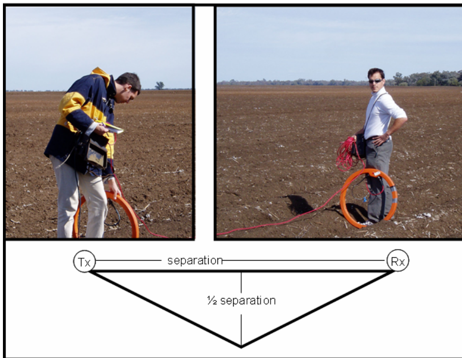
Figure 3.10. The Geonics EM 34 held in the horizontal coaxial dipole configuration, during the initial survey of the paddock. Shown below is a diagram of the instrument sampling depth of as a function of the separation distance (not to scale).
