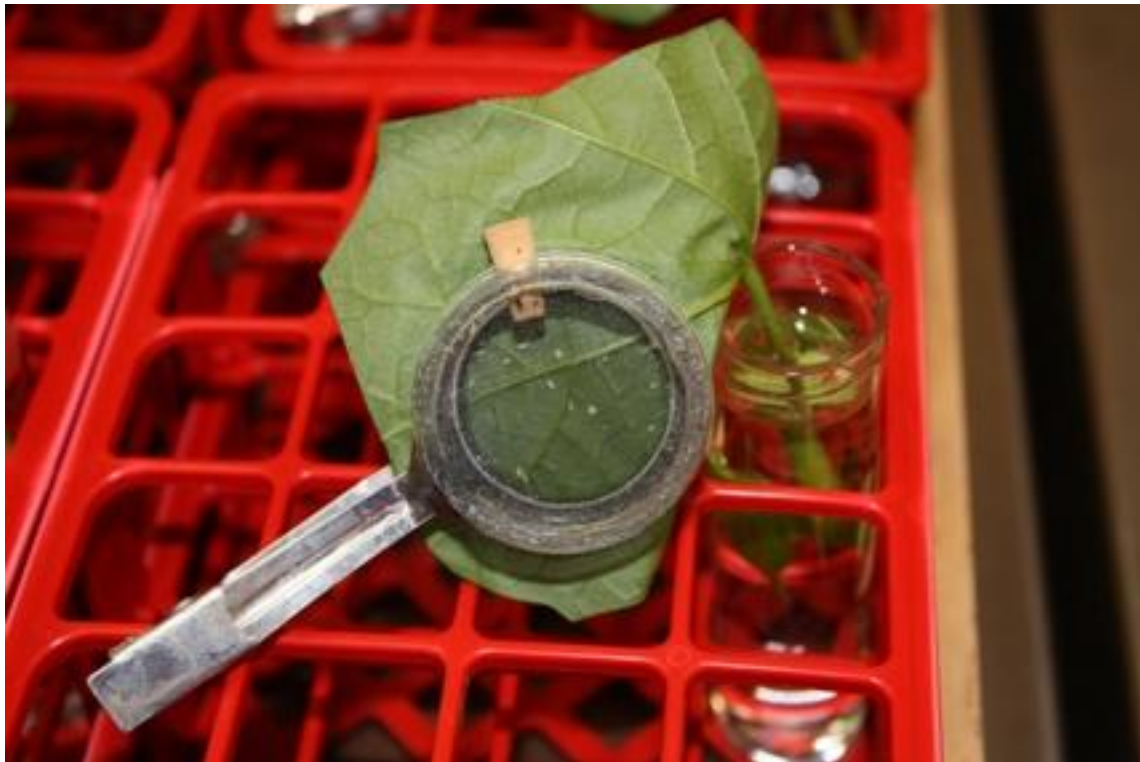
Figure 7. Clip cages developed by Steve Castle's group and optimised by Richard Lloyd, DEEDI, were used for adult SLW bioassays.
