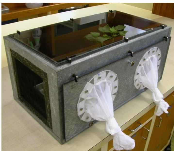
Figure 4. The emergence boxes were painted black inside with a clear glass top so that the whitefly would be attracted to the top of the cage where they could be easily removed for bioassays or be transferred to colony cages without the risk of introducing pest insects including thrips and mites.
