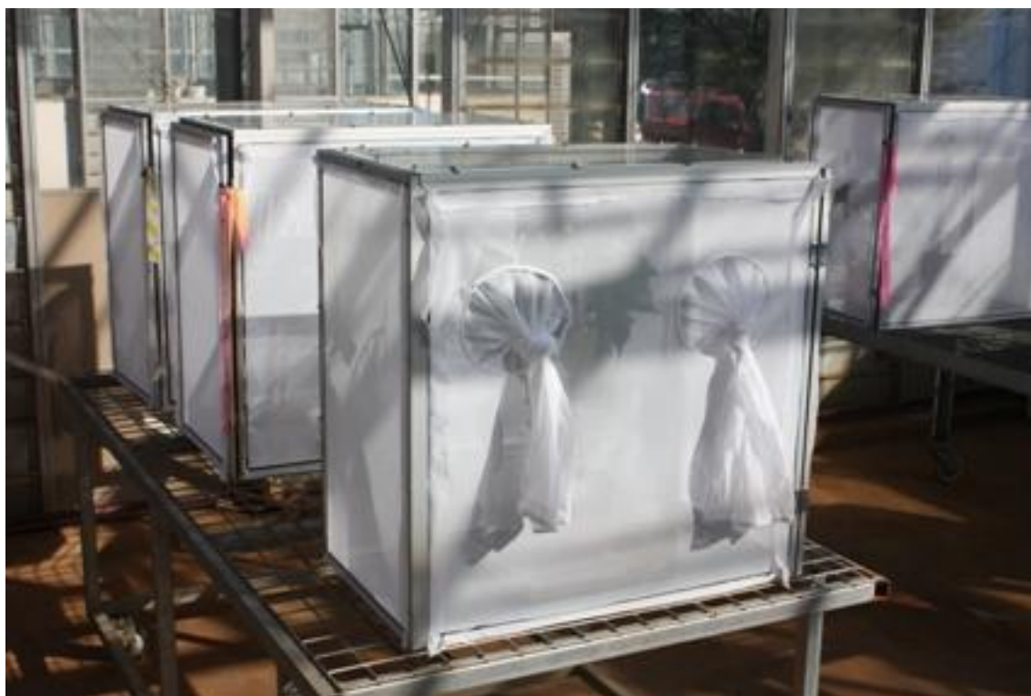
Figure 5. The colony cages were designed with light weight aluminium frames for ease of transport, insect proof netting for ventilation and a Perspex top so that insects could be easily aspirated from the roof of the cage without breaking their stylets or causing other damage.
