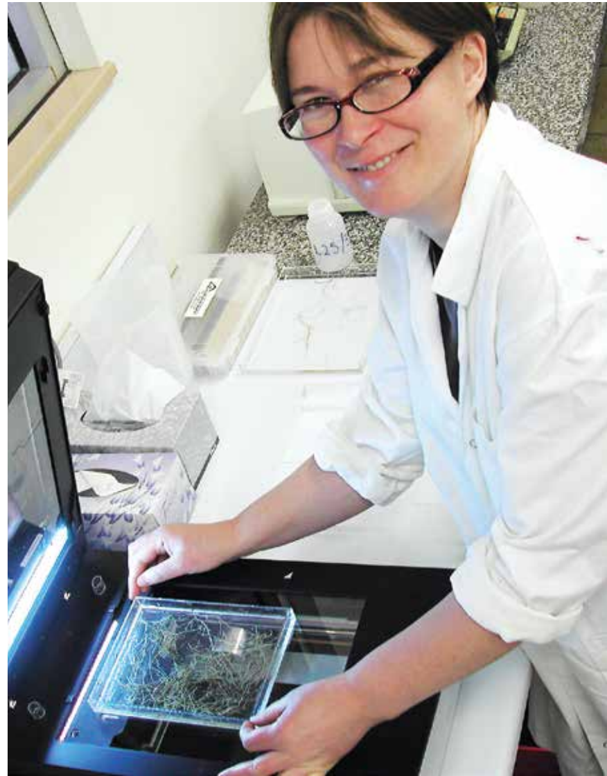
Dr Seyb washes cotton roots in preparation for analysis using the WinRhizo. The WinRhizo measures diameter, volume, surface area, length and branching of the cotton roots. It also differentiates between healthy and diseased roots saving time and sanity in the research lab and delivering precise, accurate and detailed data.
