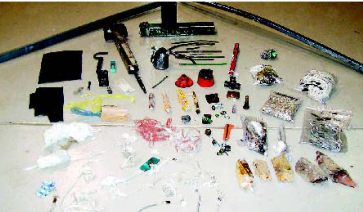
Figure 5 – Examples of contaminants collected from modules
